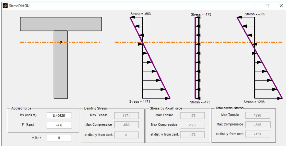
Figure 2. Stress analysis using the Secpro app
