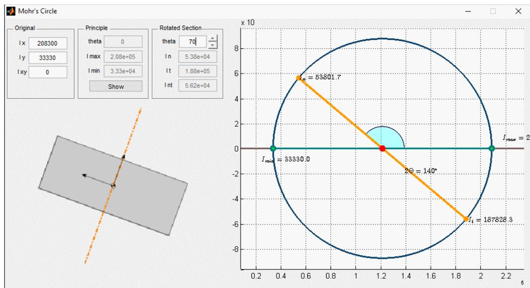
Figure 2. Rotated section and the Mohr circle in the Secpro app
